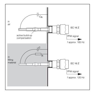
Principle of limit detection with Multicap probes
